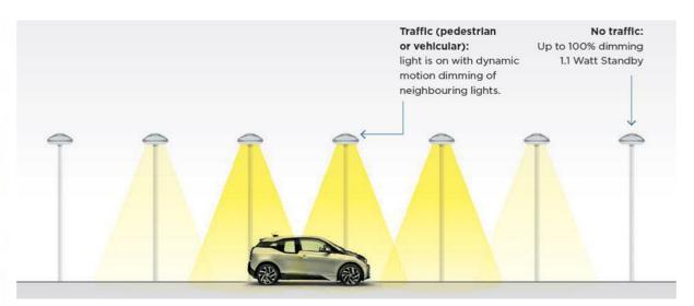
Compared to normal LED street lighting you increase energy efficiency up to 90% with the intelligent lighting system. This extends the lifetime of the luminaires and reduces maintenance costs.
